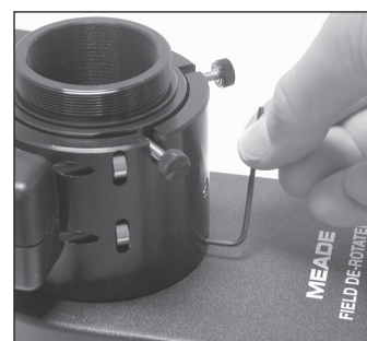
Fig. 8: Tighten the three microfocuser set screws to a firm feel.
