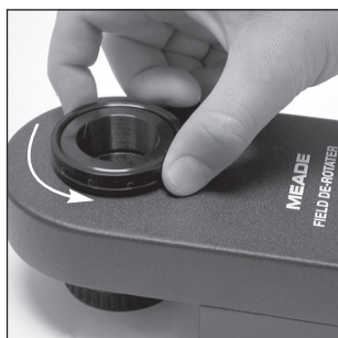
Fig. 6: Back off the adapter ring one full revolution.
