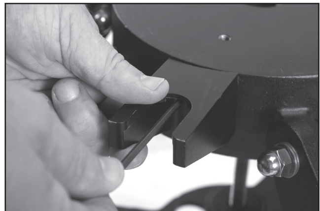
Figure D. Attach the tangent arm with the flat surface facing up.
