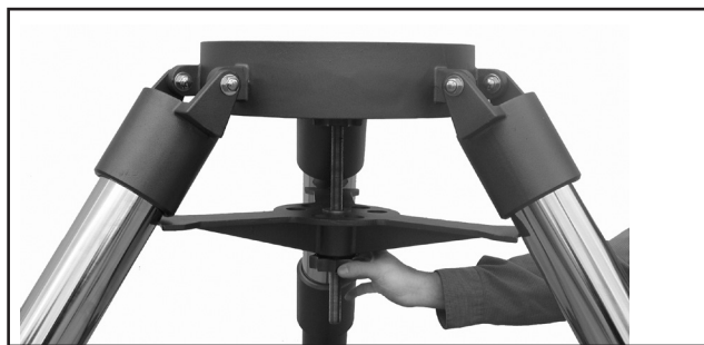
Fig. 29: Tighten the tripod spreader bar with the tension knob.
