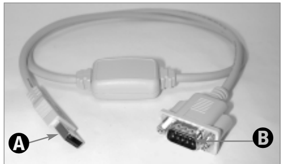
Fig. 1: The USB to RS232 Adapter cable: (A) USB connector (B) 9-pin RS232 connector.
