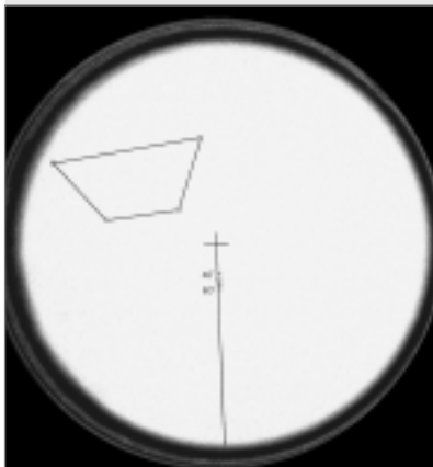
Fig. 37: The view inside the polar alignment viewfinder reticle.
