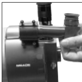
Fig. 8: Attach the viewfinder to the viewfinder bracket.
