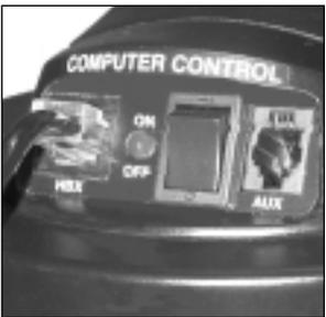
Fig. 10: Connect Autostar to the HBX port.
