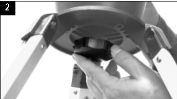
2. **Attach the mounting arm assembly:** Place the mounting arm assembly into the tripod base. Reach underneath and thread the mounting knob through the tripod base and into the mounting arm assembly. Tighten to a firm feel only, do not overtighten. While observing, you may wish to slightly loosen this knob and rotate the mounting arm assembly with attached optical tube around the horizontal axis.
