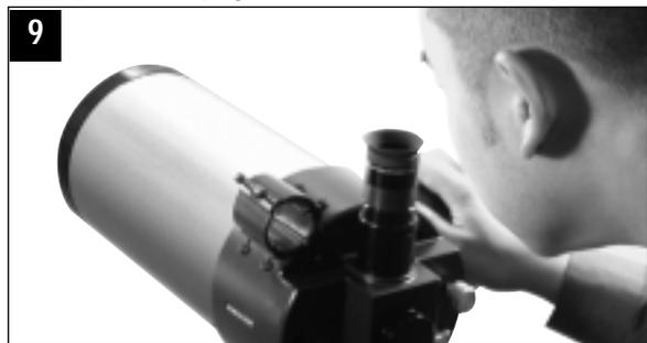
9. **Sight along the tube:** Sight along the side of the telescope's main tube to locate an object. Practice using the Autostar Arrow keys to center an object in the telescope's field of view.
