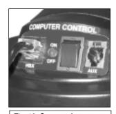
Fig. 10: Connect Autostar to the HBX port.
