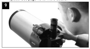
Sight along the tube: Sight along the side of the telescope's main tube to locate an object. Practice using the Autostar Arrow keys to center an object in the telescope's field of view.
