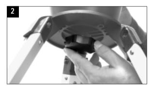
2. Attach the mounting arm assembly: Place the mounting arm assembly into the tripod base. Reach underneath and thread the mounting knob through the tripod base and into the mounting arm assembly. Tighten to a firm feel only, do not overtighten. While observing, you may wish to slightly loosen this knob and rotate the mounting arm assembly with attached optical tube around the horizontal axis.
