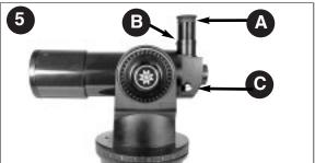
5. Tighten (to a "firm feel" only, do not overtighten) the vertical and horizontal locks (6, 9, Fig. 1). See page 5 for more information. Remove the dust cover from the end of the telescope tube. Place the MA 25mm eyepiece (A) into the eyepiece holder on the telescope and tighten the attachment thumb-screw (B) to a "firm feel" only. Make sure that the flip-mirror control (C) is in the "up" position. See page 6, for more information.
