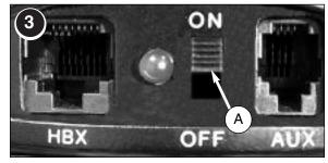
Flip the Power Switch (A) on the computer control panel to the ON position. The copyright message lights on Autostar's LCD display.
