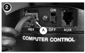
Make sure that the computer control panel power switch is in the OFF position. Remove Autostar (18, Fig. 1) from the packing materials and plug it into the HBX port (A).
