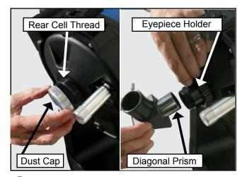
9 Remove the dust cap from the rear cell of the telescope. Thread the 1.25" eyepiece holder onto the rear cell thread. Slide the diagonal prism into the eyepiece holder and lock in place by turning the thumbscrew to a firm feel. Place the Super Plössl 26mm eyepiece into the diagonal prism and tighten the diagonal prism thumbscrew to a firm feel only.
