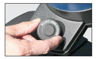
Next remove the dust cap from the ECLIPS CCD Module and put it in a safe place.
