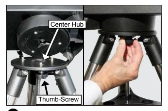
**5** Take the LS-6 from its packaging and place the entire telescope onto the top of the tripod head. Rotate the telescope head slowly until you feel the scope register on the center hub of the tripod head. Carefully screw the three attachment thumb-screws on the bottom of the plate to the base of the tripod. Hand tighten the screws so the telescope cannot spin or wobble on the tripod head.
