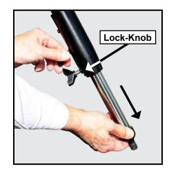
Thread in two lock-knobs on each leg (six total) near the foot of each tripod leg. Use the lock-knobs to vary the height of the inner, extendible tripod leg sections. Tighten the locks to a firm feel only; do not overtighten.
