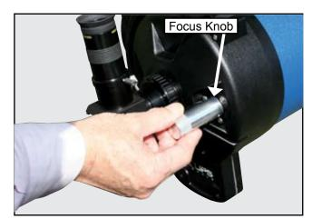
At this point look through the eyepiece of the telescope. You should see some light from the final alignment star but it is probably out of focus. Adjust the focus using the knob on the back of the telescope until you get a sharply focused star image.
