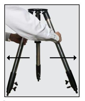
2 Remove the field tripod from the shipping carton. Stand the tripod vertically with the tripod feet down and with the tripod still fully collapsed. Grasp two of the tripod legs and, with the full weight of the tripod on the third leg, gently pull the legs apart to a fully open position.
