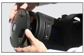
Now remove the dust cover from the front of the telescope tube. Be careful not to touch the glass lens.
