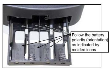
**CAUTION:** Use care to install batteries as indicated by the battery compartment. Follow battery manufacturer's precautions. Do not install batteries backwards or mix new and used batteries. Do not mix battery types. If these precautions are not followed, batteries may explode, catch fire, or leak. Improperly installed batteries void your Meade warranty. Always remove the batteries if they will not be used for a long period of time.
