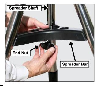
A Remove the end nut from the spreader shaft and slide the spreader in between the telescope legs. Attach the end nut and hand tighten until the telescope legs are held snuggly in the most spread position. Position the tripod where you want the telescope to be and check that the top of the tripod is approximately level.
