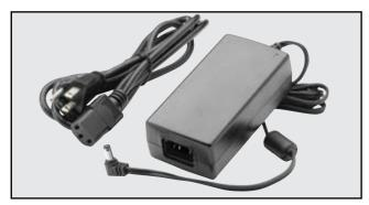
**Universal AC Adapter (07584):** This adapter supplies a constant regulated 12 volt DC at up to 5 Amps from either a standard 115 volt AC or 220 volt AC household supply. It is the only tested and recommended AC power supply for the LS-6 system.
