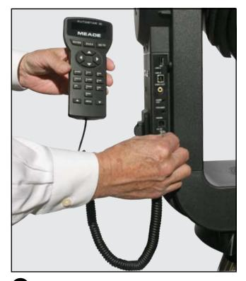
Be sure the telescope master power switch is in the off position. Remove the LS-6 handbox and the coiled interface cable from the packing materials. Plug one end into the HNDBX port of the control panel and plug the other end into the Handbox port on the LS-6 handbox.
