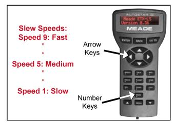
At the end of this message, the telescope will immediately start its LightSwitch Automatic Alignment procedure. It will take about five to ten minutes for the telescope to orient and align itself. Once it has completed the alignment the handbox screen will display "Alignment Successful".
