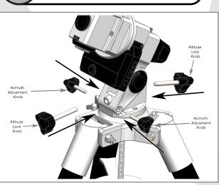
Adjust to local latitude using Altitude Adjustment and Lock Knobs
