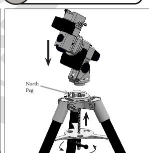
Install Latitude and Azimuth Adjustment knobs.
