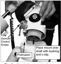
Fig. 5c: Attach the mount to the tripod.
