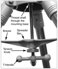
Fig. 4: Thread T-handle shaft into base. (See next page.)
