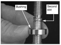
Fig. 5a: Slide bushing over shaft.
