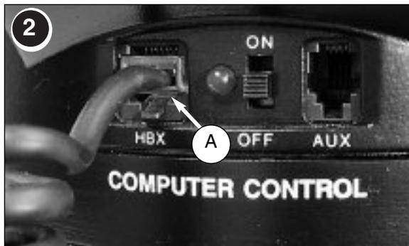
2. Make sure that the computer control panel power switch is in the OFF position. Remove Autostar (18, Fig. 1) from the packing materials and plug it into the HBX port (A).
