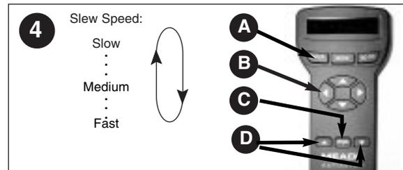
4. Press the Speed/? key (C) to accept the Sun warning. Keep pressing the ENTER key (A) until "Country/State" appears on the display. (Ignore the prompts requesting "Date" and "Time" for now – these functions will be explained later). Use the Scroll keys (D) to cycle through the lists of Country/States, Cities, and Telescope Models. Press ENTER (A) when the correct information for each prompt displays. The display then reads "Setup: Align." See page 11 for more information.
