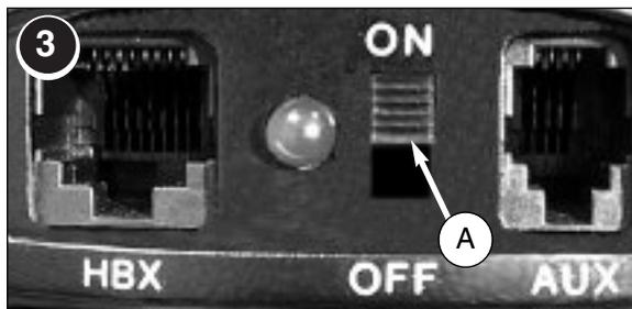
3. Flip the Power Switch (A) on the computer control panel to the ON position. The copyright message lights on Autostar's LCD display.
