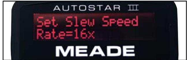
To change the telescope's speed, press the *1/SPEED* key. You can now select a speed with the scroll up and down small arrow keys on the bottom of the hand control. When you have the desired speed selected, press the "ENTER" key. Alternatively, when the speed selection screen is showing, you can just press a number 1-9 to select a speed quickly, where 1 is the slowest and 9 is the fastest.
