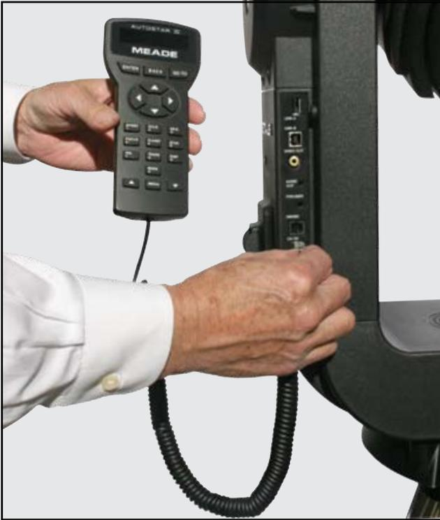
**8** Be sure the telescope master power switch is in the off position. Remove the LS-6 handbox and the coiled interface cable from the packing materials. Plug one end into the HNDXB port of the control panel and plug the other end into the Handbox port on the LS-6 handbox.
