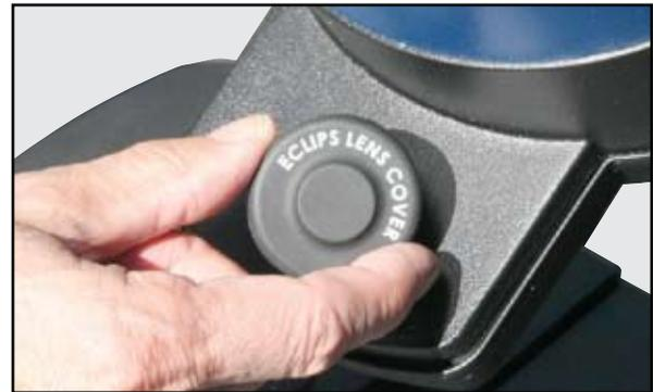
**11** Next remove the dust cap from the ECLIPS CCD Module and put it in a safe place.
