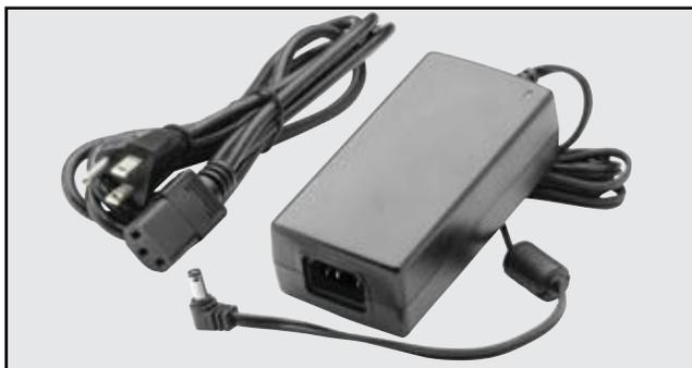
**Universal AC Adapter (07584):** This adapter supplies a constant regulated 12 volt DC at up to 5 Amps from either a standard 115 volt AC or 220 volt AC household supply. It is the only tested and recommended AC power supply for the LS-6 system.
