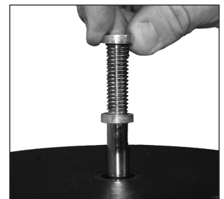
Fig. E, 2: Thread the first nut as far down as it will go. Then thread the second nut down onto the first nut.
