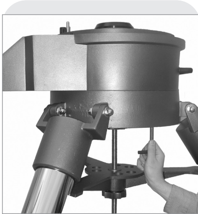
Fig. 50: Attach the drive base to the tripod.
