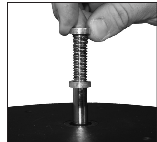
Fig. G: Thread the first nut as far down as it will go. Then thread the second nut down onto the first nut
